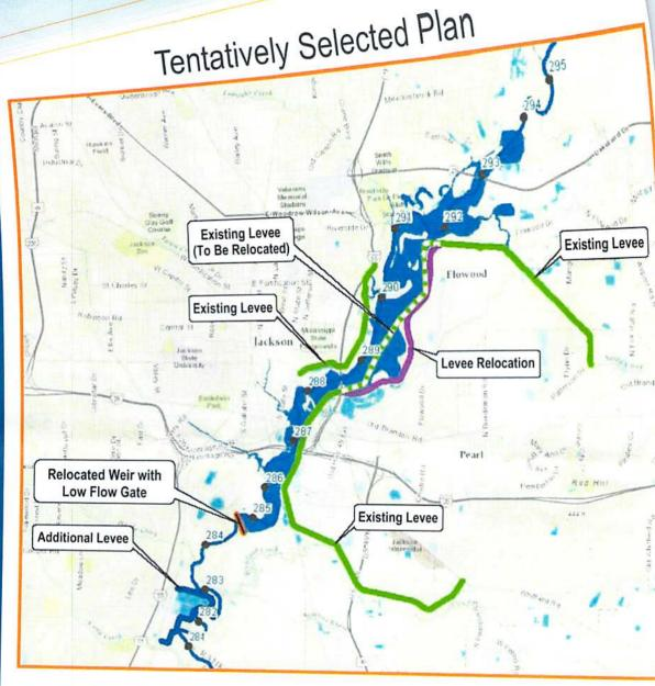
The Tentatively Selected Plan for bringing substantive flood risk management to the Jackson Metropolitan Area is a combination of excavating and widening the Pearl River while reinforcing the existing levee system. It also includes relocating and improving an existing weir to a location just downstream from I-20.
